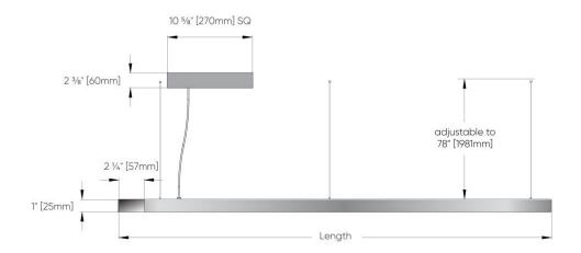
Canopy: 12" [305mm] SQ [for a total of 107W combined for direct/Indirect] Note: The diffuser protrudes by  $^3/_{16}$ " [5mm]
