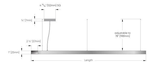
Note: The diffuser protrudes by  $\frac{3}{16}$ " [5mm]
