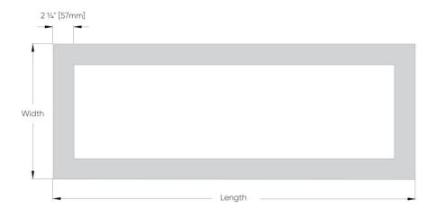
Note: The diffuser protrudes by  $^3/_{16}"$  [5mm]
