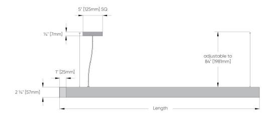
Note: The diffuser protrudes by  $\frac{3}{16}$ " [5mm]
