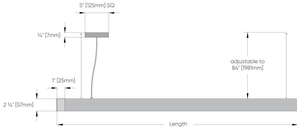
Note: The diffuser protrudes by  $3/16$ " [5mm]
