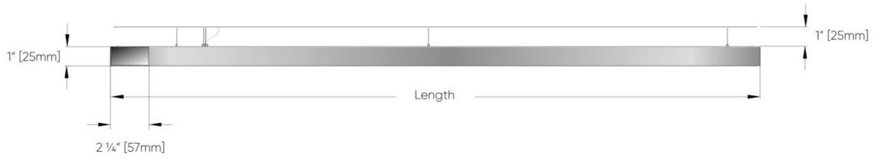
Note: The diffuser protrudes by 3/16" [5mm]
