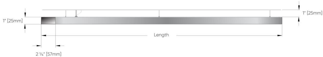
Note: The diffuser protrudes by 3/16" [5mm]
