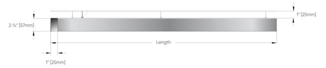
Note: The diffuser protrudes by 3/16" [5mm]
