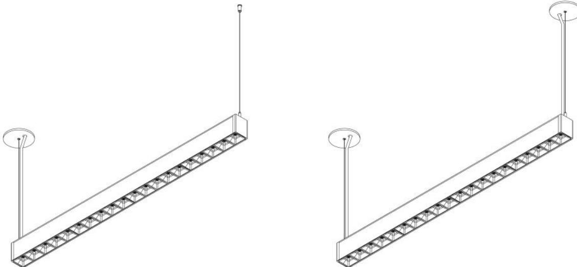
2 Power feeds will be necessary in the case that Direct/Indirect illumination is requested with Tunable White Direct option.
