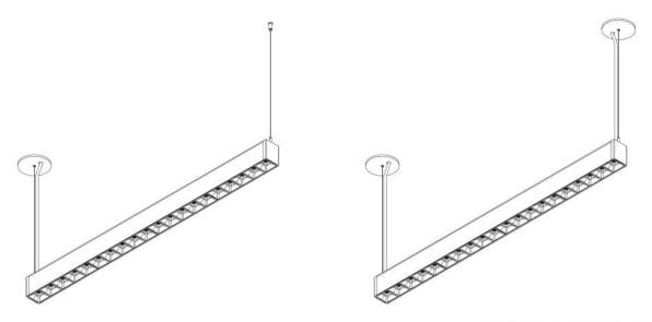
2 Power feeds will be necessary in the case that Direct/Indirect illumination is requested with Tunable White Direct option.
