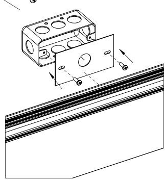
4. Install fixture into the wall bracket and secure in position using the provided screws.
