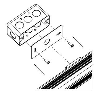
4. Install fixture into the wall bracket and secure in position using the provided screws.
