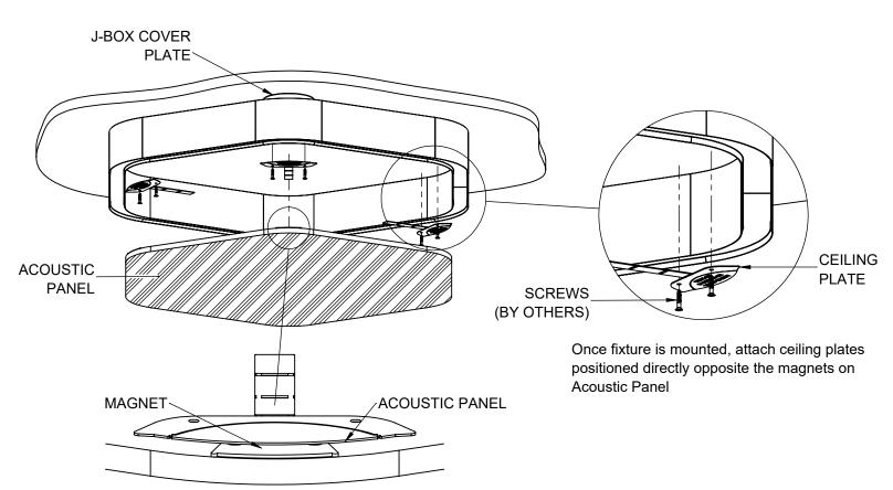
One magnet position will use the J-BOX cover plate as its mounting point
