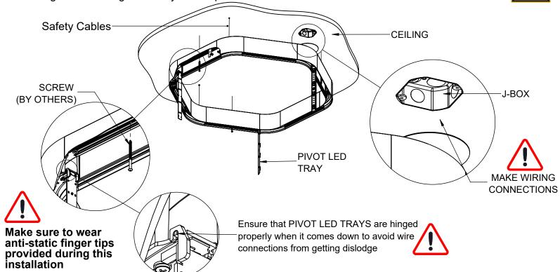
Reinstall pivot LED trays and make sure to place a nylon washer between the screws and LED board. Mount the diffusers back with textured surface facing outwards
