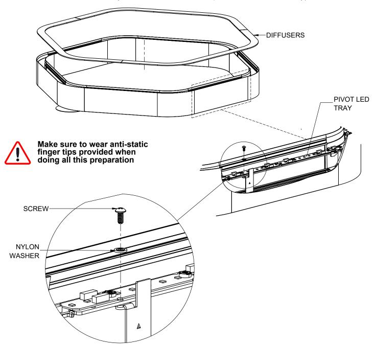
Remove screws that secures the pivot gear trays. On **page 5**, check for the recommended mounting hole locations for each corresponsing fixture size (NOTE: Only perform these on tray assemblies that directly covers the mounting holes).
