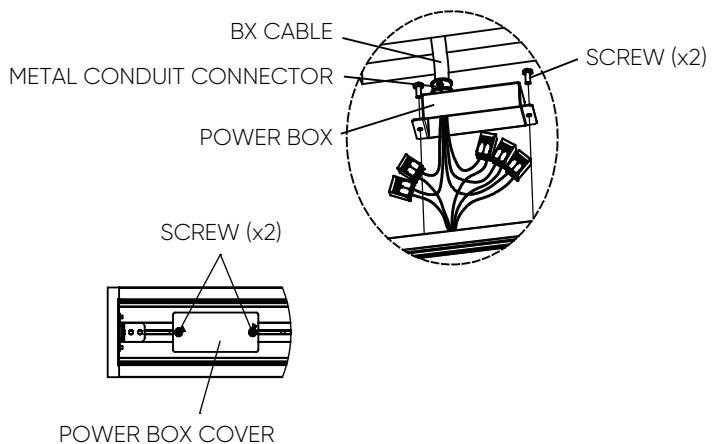
To gain access inside the power box when the fixture is installed on the ceiling, remove the power box cover inside the fixture by loosening two screws.
