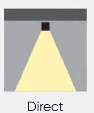
Illuminate interiors with focused beams, ideal for accentuating artwork or creating task-oriented environments.
