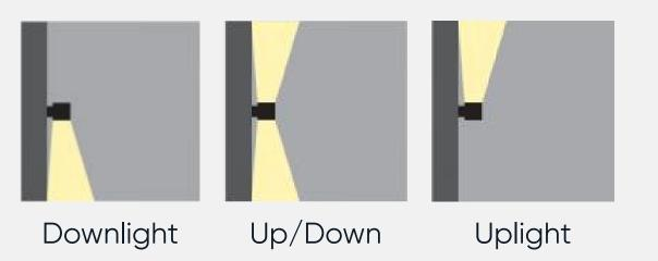
Illuminate architectural features while enhancing visibility and safety on adjacent sidewalks, pathways, or parking lots. Harness the versatility of multiple light distributions to target specific tasks without overlighting while ensuring minimal light spill.
