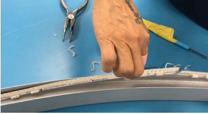
Remove the defective LEDs
