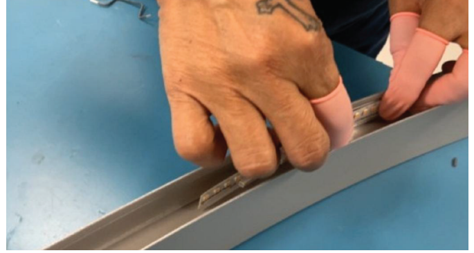
Place the new LEDs in the frame
