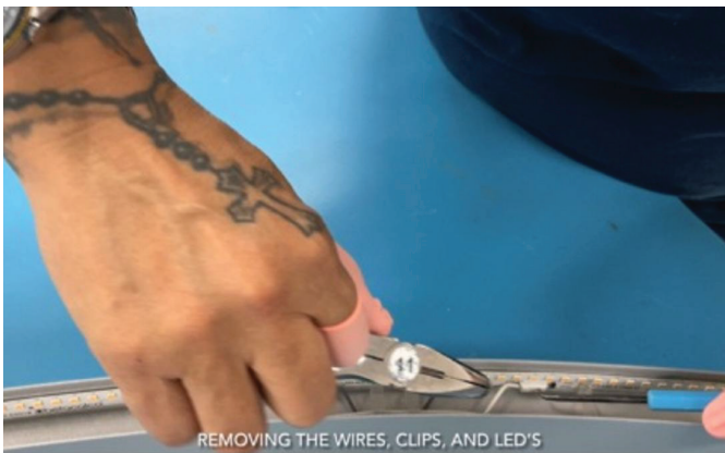
Using angle long nose flyer and angle pointed hook tool, remove the wires connected to the small terminal block of the LED. NOTE: USE A FINGER CLOTS WHEN HANDLING THE LEDs
