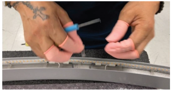
Insert the clips to secure the end portion of the LEDs
