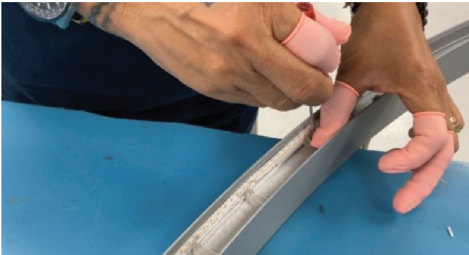
Insert the clips to secure the LEDs in place
