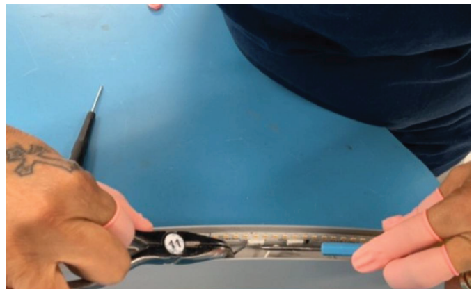
Place the pointed portion of the angle pointed tool to the small hole of the terminal block and carefully remove the wire by angle longnose flyer
