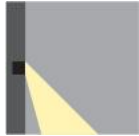
Ext-Wall Recessed Downlight
