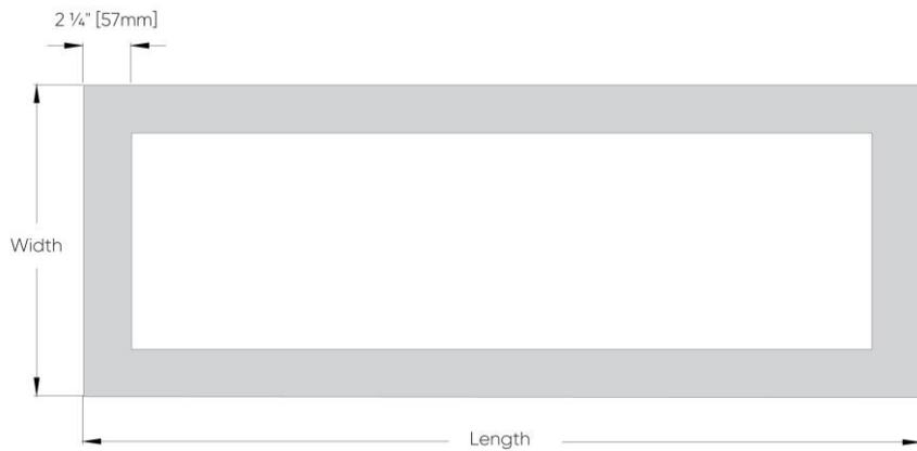
Note: The diffuser protrudes by 3/16" [5mm]
