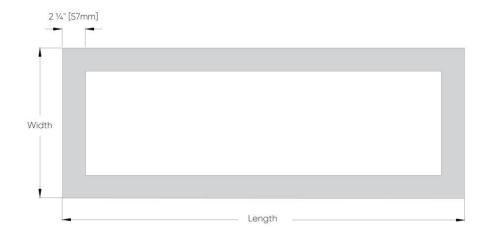
Note: The diffuser protrudes by  $^{3}\!/_{16}"$  [5mm]
