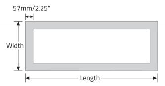
Note: The diffuser protrudes by 4.8mm/0.19"
