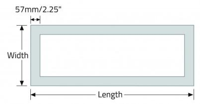
Note: The diffuser protrudes by 4.8mm/0.19"
