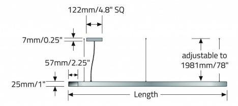
Note: The diffuser protrudes by 4.8mm/0.19"
