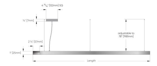
Note: The diffuser protrudes by  $^{3}\!/_{16}"$  [5mm]
