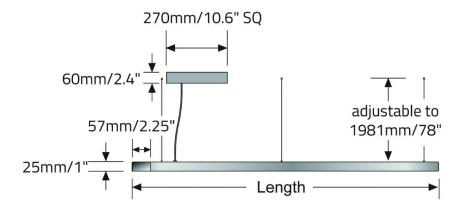
**Canopy:** 305mm/12" SQ (for a total of 107W combined for direct/Indirect) **Note:** The diffuser protrudes by 4.8mm/0.19"
