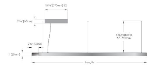
Canopy: 12" [305mm] SQ [for a total of 107W combined for direct/Indirect] Note: The diffuser protrudes by  $^{3}{\prime}_{16}$ " [5mm]
