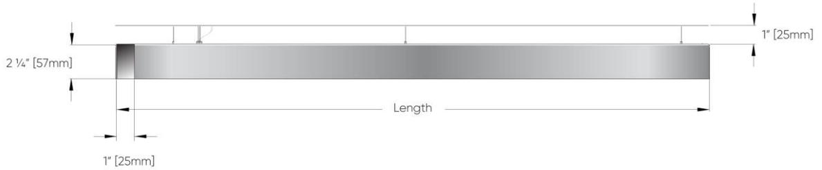
Note: The diffuser protrudes by 3/16" [5mm]
