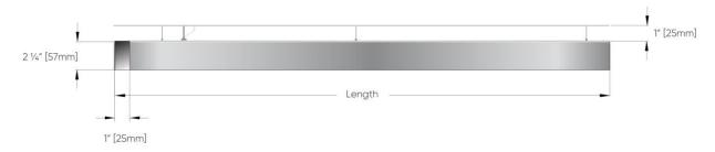
Note: The diffuser protrudes by 3/16" [5mm]
