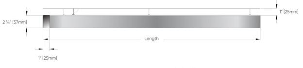
Note: The diffuser protrudes by 3/16" [5mm]
