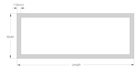
Note: The diffuser protrudes by  $^{3}/_{16}"$  [5mm]
