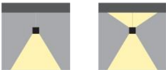
Suspended Direct Suspended Direct/Indirect
