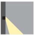
Ext-Wall Recessed Downlight
