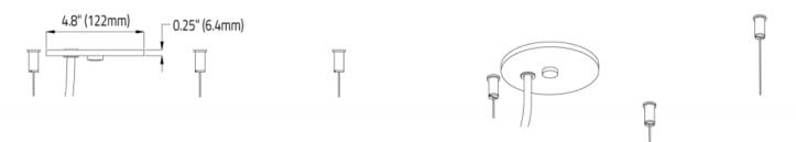
**CN1 (Canopy A)** Drivers are Integral within the fixture, not available with RGBW or TRPP2P06 when ordering 1400 lms direct. **CN3 (Canopy C)** Drivers are in the remote box and can be used with RGBW for both NA & EU.
